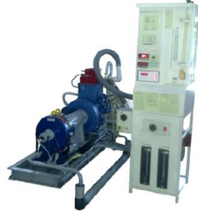
Fig.1 4-Stroke, Single Cylinder Diesel Engine Test Rig
