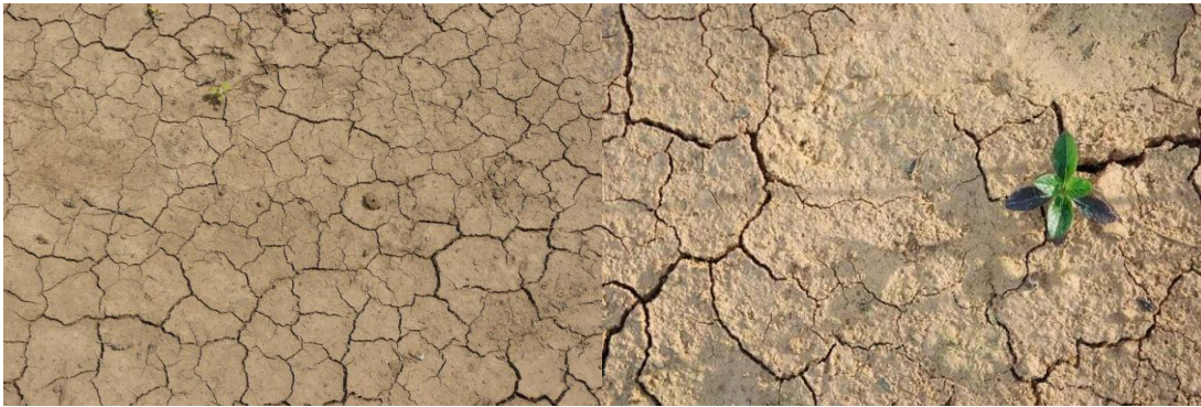
Figure: 2 Soil Expansion/Shrinkage
