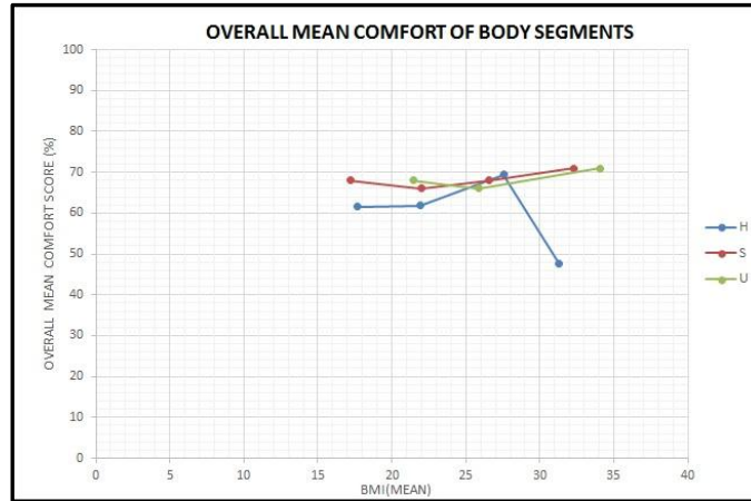
Fig. No. 5: Comparison of Overall mean comfort of body segments with type of car and BMI (H: Hatchback S: Sedan U: SUV)
