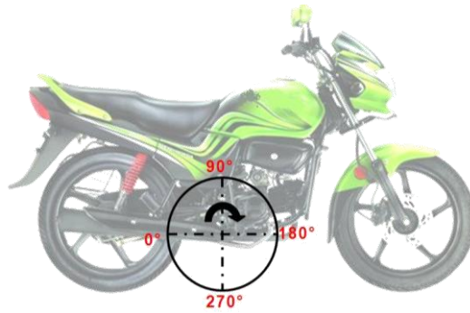
Fig.3 Exhaust opening angle configuration
