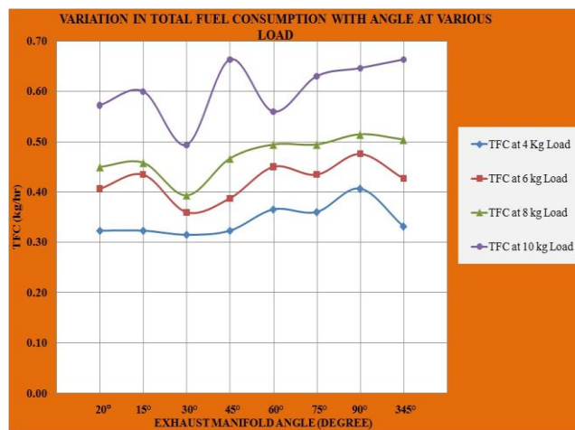
Fig.7 Variation in TFC with Manifold Angle for 3000 RPM
