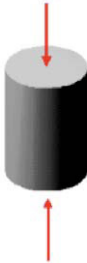
Fig.7 Uniaxial Test on Concrete Cylinder ASTM C-39
