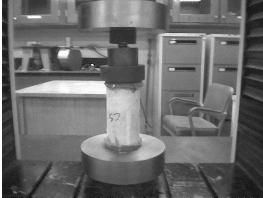
Fig.4 Compressive Strength Testing
